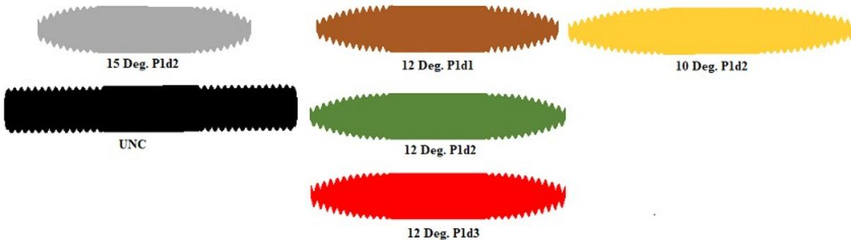
variety of wave threaded 5/8" (15.6mm) nuts and studs; and standard UNC threaded nut and stud. They were 3D printed on site with a nylon/carbon fiber material mix. The colors align parts with the following graph lines. It is very clear that the 25% greater
