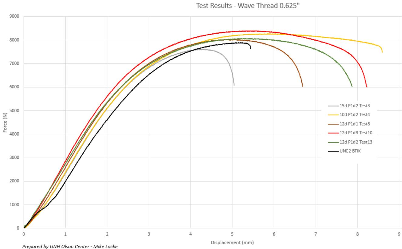
I believe the wave threaded connections can approach the strength of a solid shaft. That was not proven here. What is needed are metals. I have made the nut and stud STL files available to anyone who is interested in selling stronger fasteners. The objective is proof of concept with destructive test. These files can be used in Finite Element Analysis.
